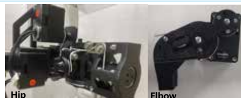
Fig5. Photo of the current prototype. The structure is entirely 3D-printed using PLA. The rope has a diameter of 1.2 mm and a load capacity of 45 kg.
