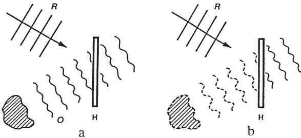
spherical wave (-1st order diffraction). Besides the virtual image at the original position of the object, there is also a real image on the other side of the hologram.
