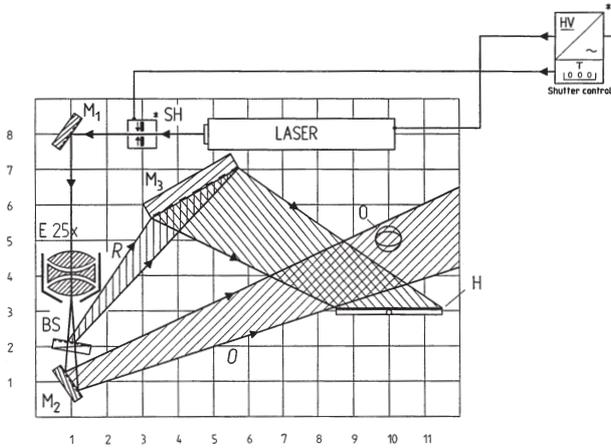
Fig. 8: Setup for recording a white light reflection hologram.
