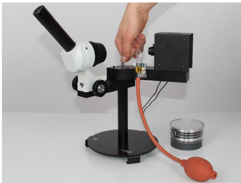
Fig. 2 : Adjustment of focus with thumb.
