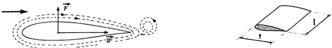
Fig 4 : Illustration of forces on a wing a wing.
