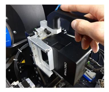
**Note:** sample alignment can be automated by using a predefined script when launching the measurements. However, manual alignment is usually faster and possible problems can be spotted quicker. It is suggested to align manually, and when screening multiple samples saving aligned motor positions for each sample into a job file. If you want use automated alignment and do not know how to please get in touch with the facility.
