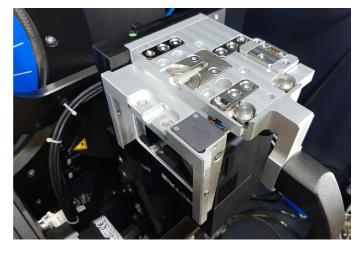
D. Unfasten the latch on the back of the track by pulling it the left with your fingers. The little circle shows green when it is locked and red when it is free. CAREFUL. When you have unfastened you will feel weight on the handle, the magnet supports the detector but does not hold it in place.
