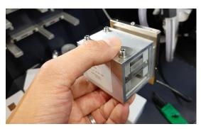
Touch the mirror at top and bottom only, and carefully fasten it with the snap-lock mechanism on the track, as all other optics that you mount directly on the track (those in white boxes).
