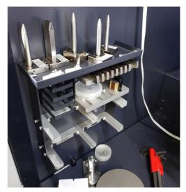
**Secondary side optics** and covers/optics for detector are stored on the right-hand side.
