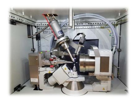
Rigaku Supernova 2 micro-sources, CCD detector, kappa goniometer, low temperature device
