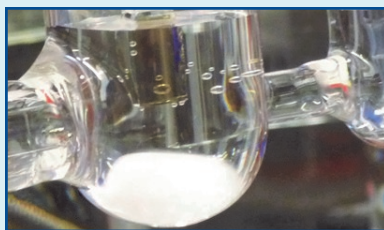
Catalytic H 2 production (bubbles) from water
