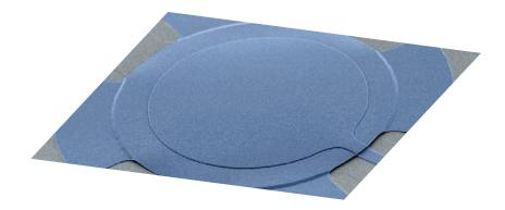
PFL researchers use a mechanical micrometre-size drum cooled close to the quantum ground state to amplify microwaves in a superconducting circuit.
