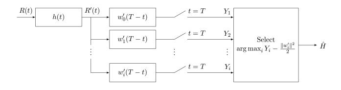
Let  $N'(t) = \int N(\alpha)h(t-\alpha) \ d\alpha$  be the noise at the output of the whitening filter. We want to select the filter h(t) such that  $\frac{N_0}{2} = G(f)|h_{\mathcal{F}}(f)|^2$ , i.e.,
