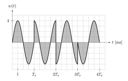
The figure above shows a toy passband signal. (Its carrier frequency is unusually low with respect to its symbol rate.) Specify the three layers of a transmitter that generates the given signal, namely the following:
