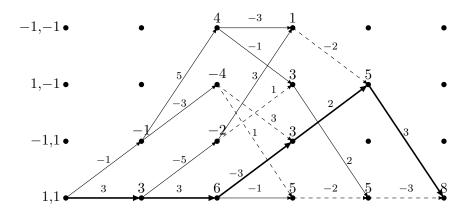
From the figure we can read the decoded sequence 1, 1, -1, 1, 1.
