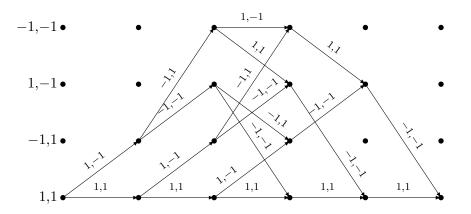
We display the diagram labeled with edge-metric according to the received sequence and state-metric of the survivor path. We also indicate the survivor paths and the decoding path.
