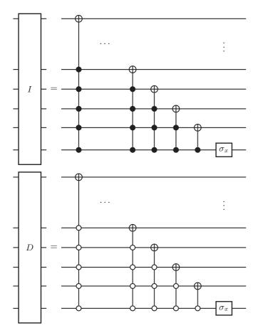
FIG. 2. Circuit diagram for the increment and decrement operators acting on qubits storing the data for a given dimension (the set of  $n_a$  qubits). This implementation is borrowed from [60].
