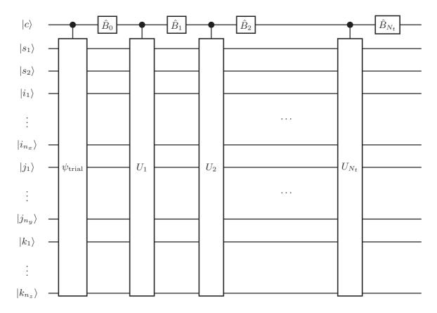
FIG. 10. Circuit diagram for the quantum implementation of the Feit-Fleck method. The gate  $U_i := U[(i-1)\Delta t, i\,\Delta t]$  advances the solution by  $\Delta t$  and its decomposition into quantum gates is given in Fig. 4. The gate  $B_i$  is defined in Eq. (D10).
