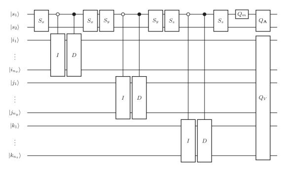
FIG. 4. Circuit diagram that evolves the wave function by one time step. The details of the spin rotation gates  $H_a|_{a=x,y,z}$  are given in Fig. 1 and Eq. (46). The increment and decrement operators I and D, respectively, are detailed in Fig. 2 and Eqs. (47)–(52). The mass operator  $Q_m$  is given in Eq. (54). Finally, the operator  $Q_A$  is displayed in Fig. 3 and is explicitly written in Eqs. (58)–(63).
