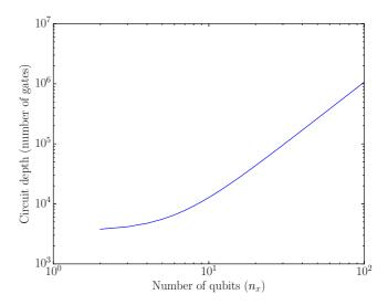
FIG. 5. Circuit depth (number of gates) required to evolve the wave function by one time step as a function of the number of qubits. The number of qubits corresponds to  $n_x$ . It is assumed that  $n_x = n_y = n_z$ . The circuit width required is then given by  $n_{\text{total}} = 4n_x + 2$ .
