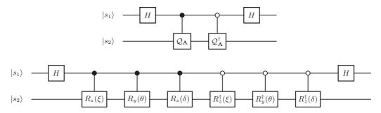
FIG. 3. Circuit diagram that implements the local operator  $Q_A$ . The bottom picture displays explicitly the decomposition of the matrices  $Q_A$  and  $Q_A^{\dagger}$ , appearing in the top picture.
