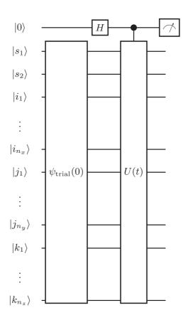
FIG. 9. Circuit diagram for the computation of the autocorrelation function. The quantity  $\langle (\sigma_x + i\sigma_y) \otimes \mathbb{I} \rangle$  is measured on the ancilla qubit.
