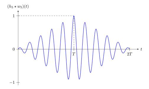
Note that the resulting signal is zero for  $t \leq 0$  and also for  $t \geq 2T$ . The figure also reveals why sampling at time t = T is a good idea: the value of the matched filter output signal is maximal.
