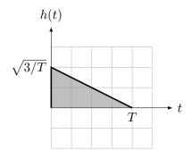
The output of the matched filter sampled at t=T and  $t=T+T_d$  is  $Y_1=\langle R(t),\frac{w_1(t)}{\|w_1\|}\rangle$  and  $Y_2=\langle R(t),\frac{w_2(t)}{\|w_2\|}\rangle$  respectively. The decision rule is
