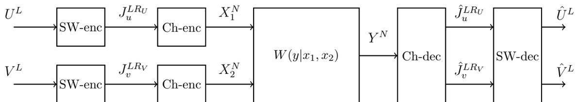
Here, SW-enc represents Slepian-Wolf encoder for the source  $U, V$  of length  $L$  which outputs a bitstream of length  $LR_U, LR_V$  respectively. Later, the bitstreams  $J_u$  and  $J_v$  are encoded by channel encoders (Ch-enc) and then passed through the multiple access channel. As usual, from  $Y^N$ ; bitstreams  $\hat{J}_u$  and  $\hat{J}_v$  are estimated by a channel decoder. Finally, the estimated bitstreams are decoded by Slepian-Wolf decoders to obtain  $U^L$  and  $V^L$ .
