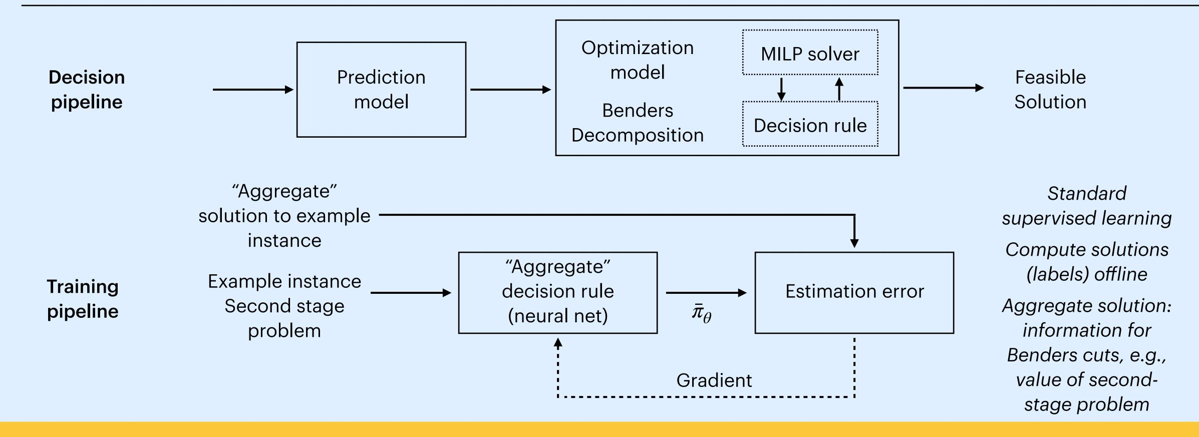
Feasibility guaranteed because general purpose solver is used at deployment. Speed ups of one to two orders of magnitude and optimality gaps close to zero.
