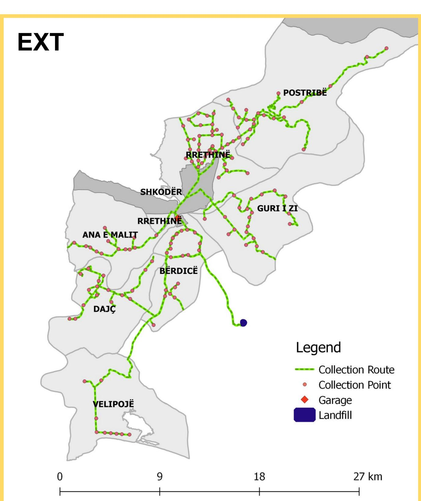
Figure 3: Overview of truck itinerary and placement of collection points in the BAU (left), OPT (middle), and EXT (right) scenarios.
