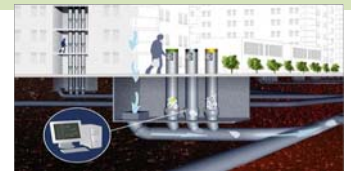
Aspiration in tubes under vacuum avoiding disturbances of dump trucks
