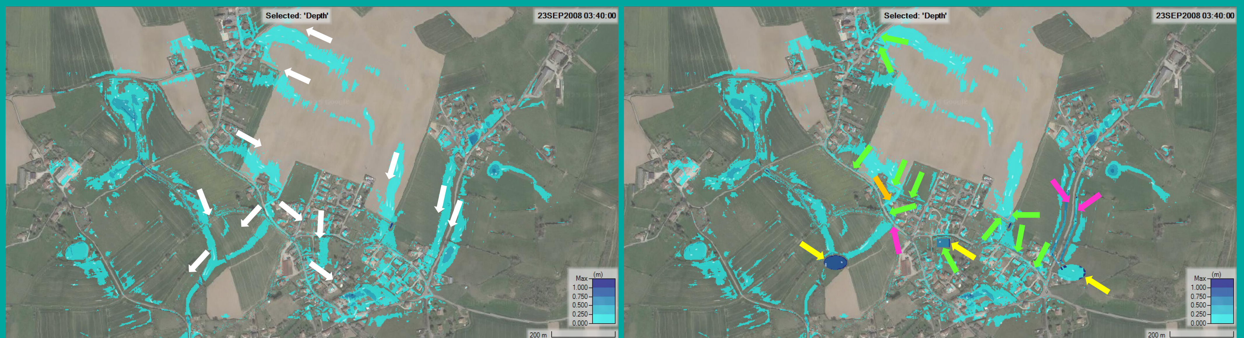
—> Flow direction —> Retention pond —> Vegetated ditches —> Fascines/hedges —> Permeable pavement Fig: Simulated water depth across the project area without (left) and with (right) NBS applied, shown in blue shades. White particles indicate flow direction.
