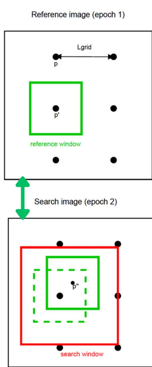
A template-based algorithm is applied between the reference window -around  $p'$ - and a subregion of the search window -around  $p''$ - to quantify the correspondence between the two areas. The displacement is then  $p'' - p'$ . It defines the magnitude and the orientation of the resulting velocity vectors.
