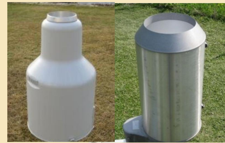
[Pluviometers: 1518 H3 e 15188 Lambrecht and Pluvio2[1]]
