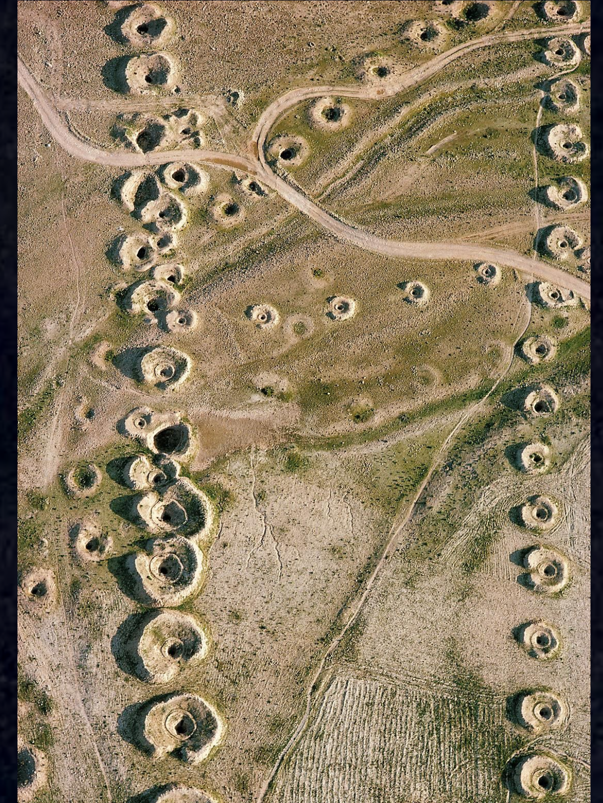
Unqanat, an ancient Persian underground water supply and irrigation system, Iran
