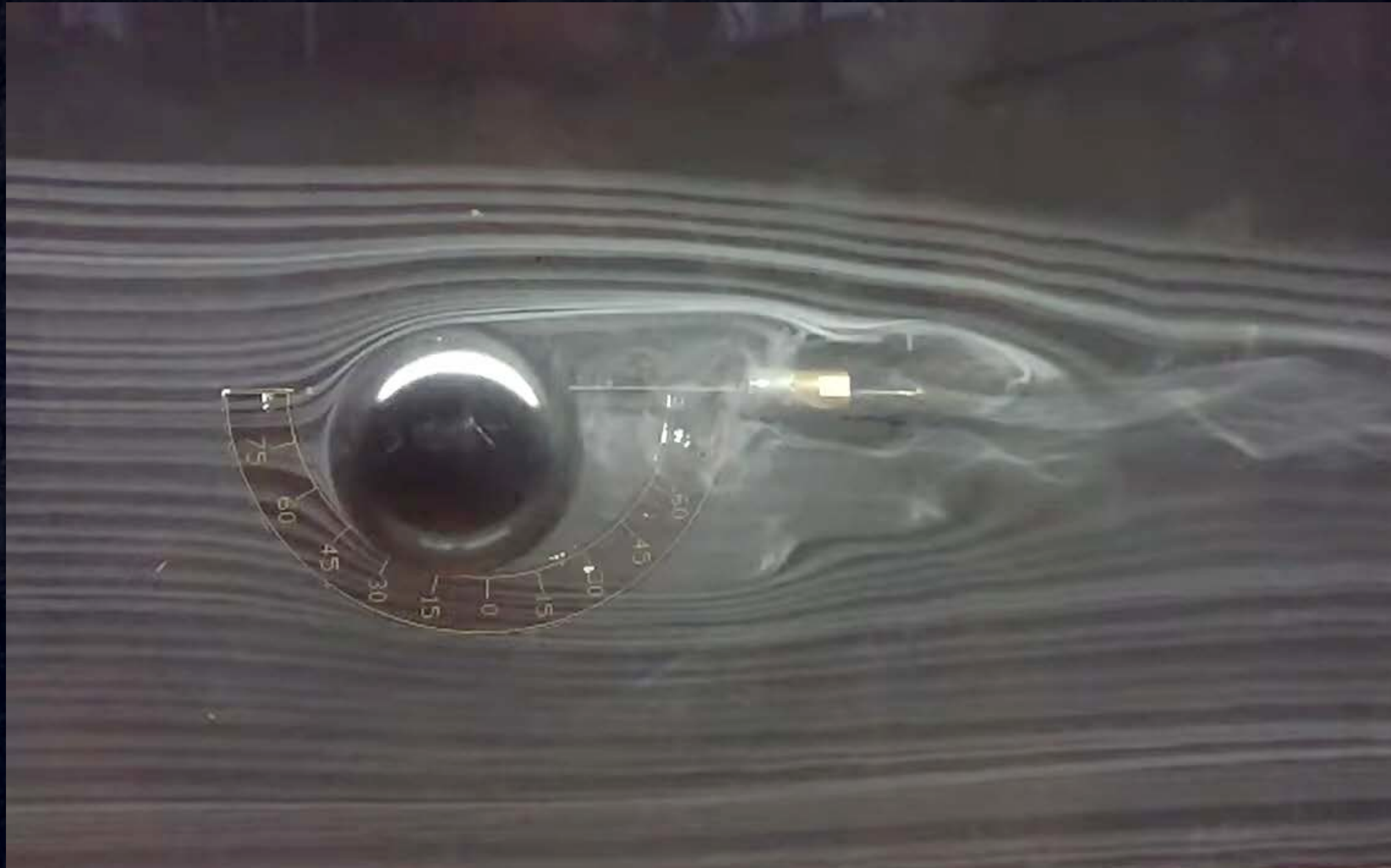
Wind tunnel smoke test displaying laminar and turbulent airflow (streamlines) passing a sphere
