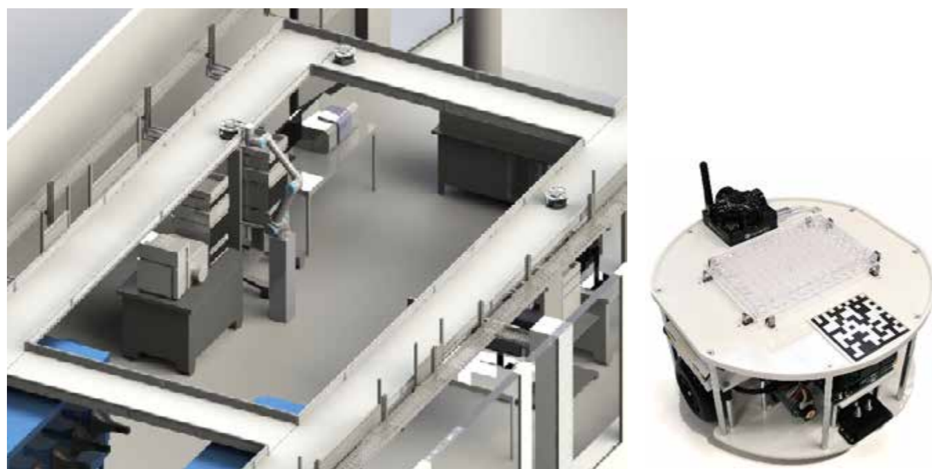
Figure 23 : Left, the dedicated track on top of the scientific equipment with the UR robots used to transfer the sample between the mini-robots and the equipment. On the right, an image of the actual 3D printed robot (25 cm diameter, 2 kg, < 1 kCHF / robot) with a standard 96 well SBS plate. The robot is located using an ultrasonic GPS (Marvelmind) and the robot is identified and precisely aligned using the QR code and a set of industrial cameras.
