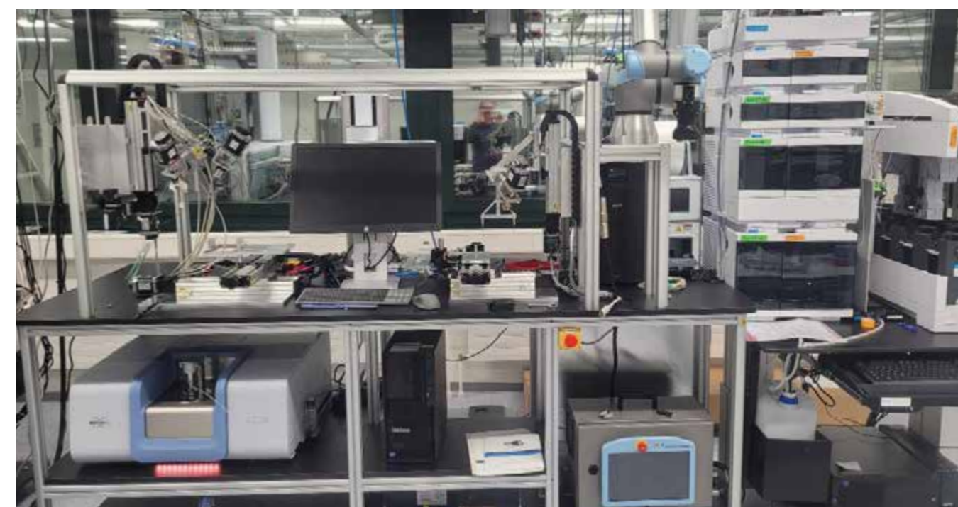
management capabilities from the RapidFire with new NMR sample preparation and on-line optical spectroscopy. On the right, we can see the actual version of the OmniFire currently being finalized.
