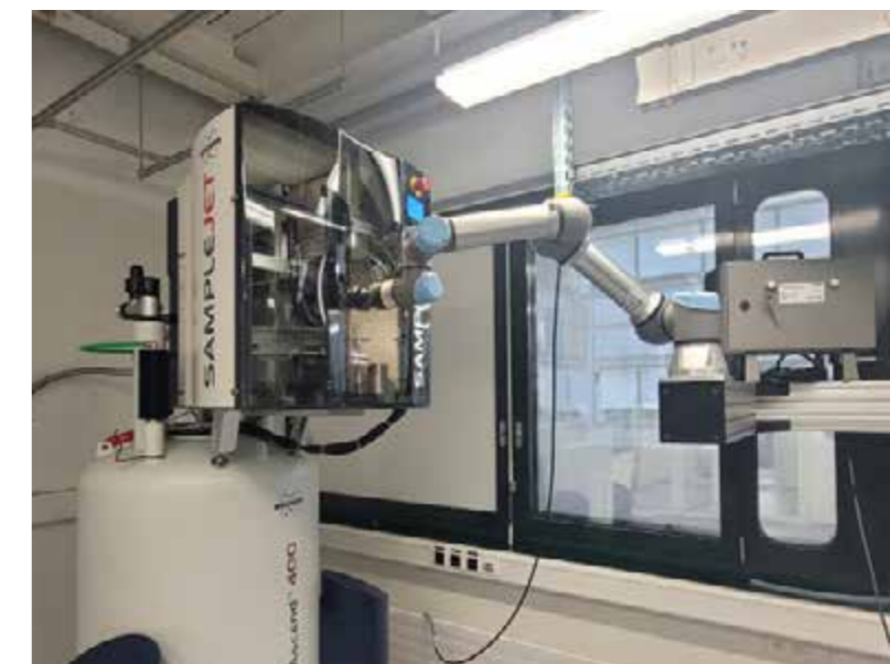
Figure 21 : A robotized Bruker 400 MHz NEO NMR spectrometer equipped with a SampleJet autosampler. The six-axis robotic arm is a Universal Robot UR5e piloted through the laboratory scheduler and connected to the NMR with dedicated libraries.
