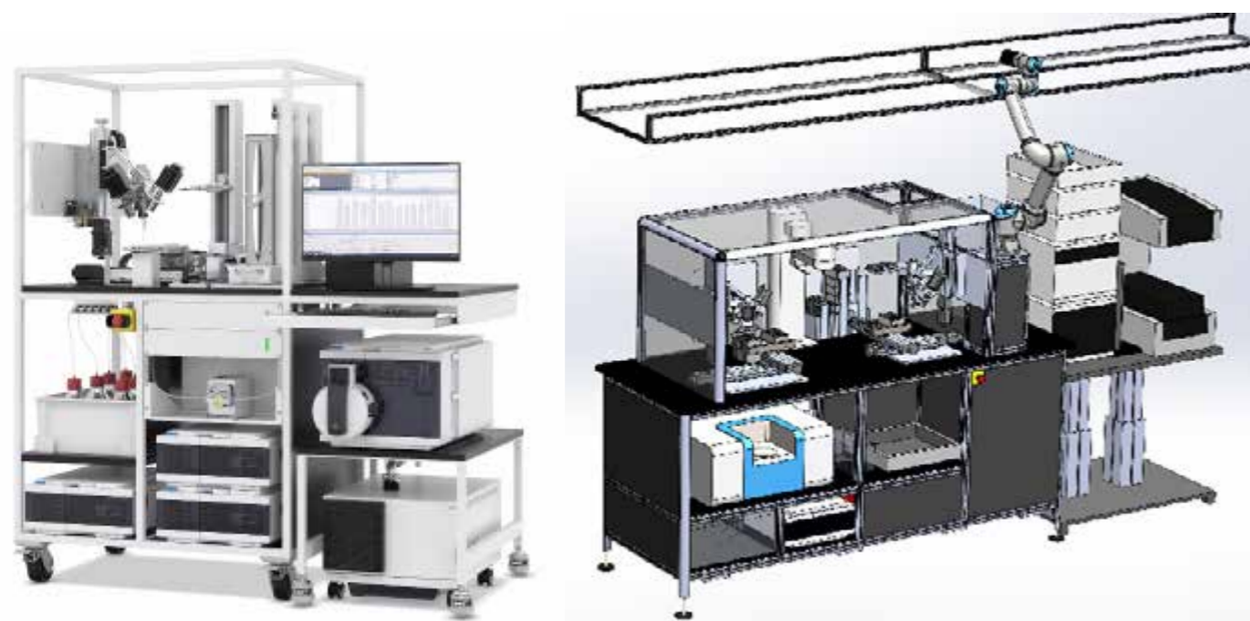
Figure 22 : From left to right, the commercially available Agilent OmniFire. Then in the center we can see the CAD rendering (SolidWorks) for the enhanced version of the original RapidFire from Agilent locally called OmniFire. It is designed to combine the initially existing high-throughput sample preparation and solvent
