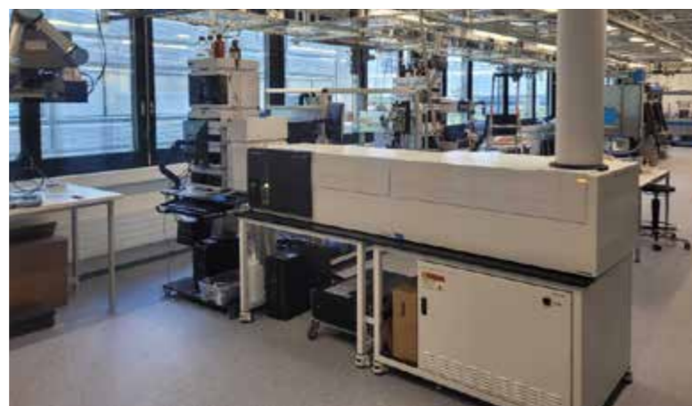
Figure 16 : Agilent SFC-IM-Q-TOF for ion mobility (CCS) determination and high-resolution mass spectrometry.IT architecture and data-driven strategy
