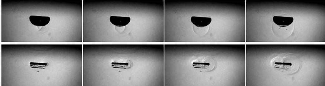
FIG. 2. Shadowgraphy visualizing the shock waves emitted as a result of the jet impact (upper row) and the toroidal collapse (lower row). Interframe time 300 ns and exposure 50 ns.
