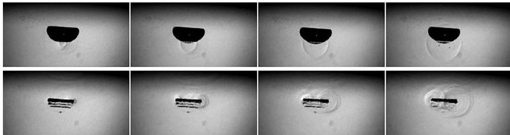
FIG. 2. Shadowgraphy visualizing the shock waves emitted as a result of the jet impact (upper row) and the toroidal collapse (lower row). Interframe time 300 ns and exposure 50 ns.
