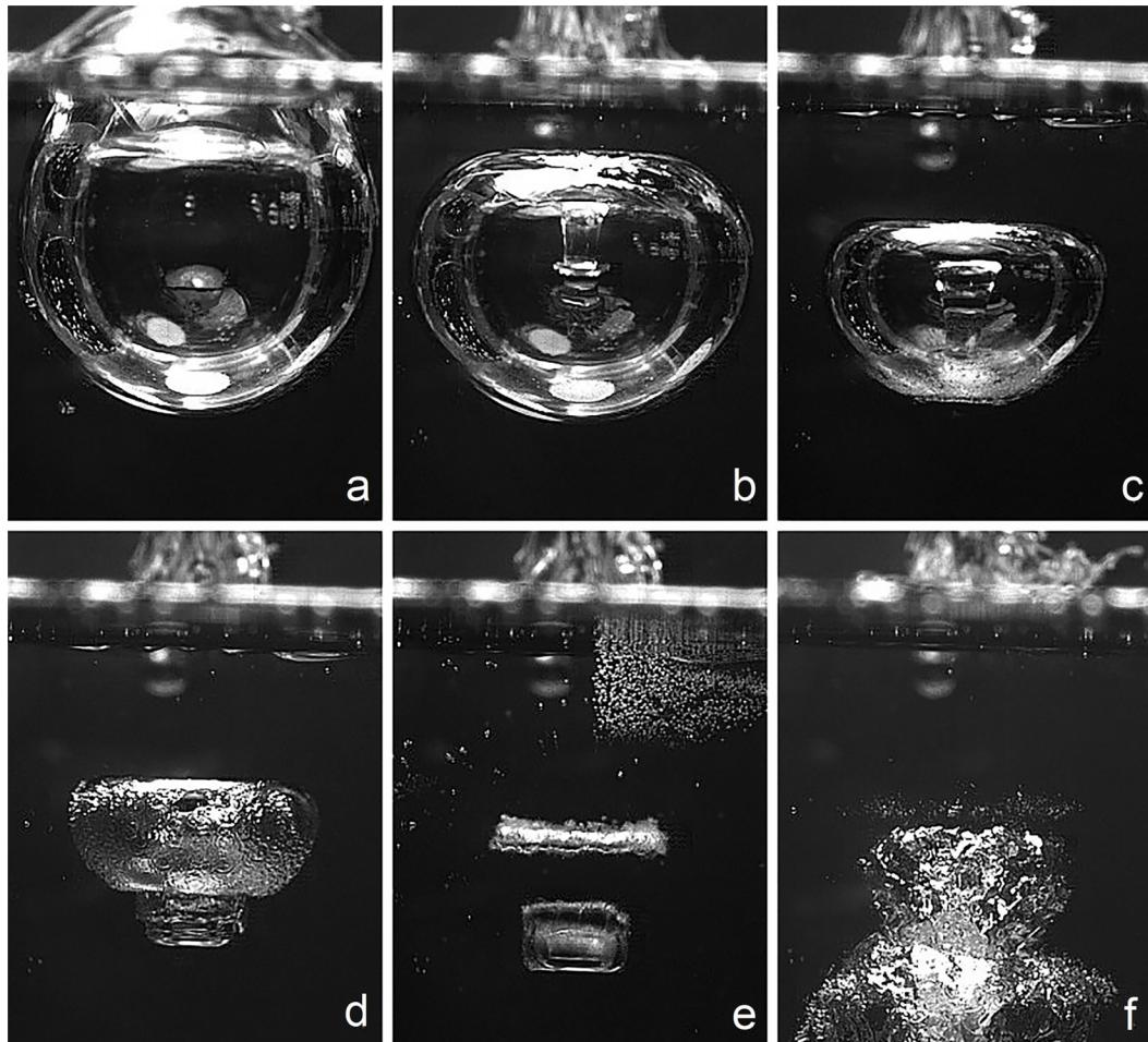
FIG. 1. A centimetric cavitating bubble collapsing in the vicinity of a free surface is pierced by a liquid microjet. The snapshots are shown from instants (a)  $t = 0$ , (b)  $t = 0.3t_c$ , (c)  $t = 0.5t_c$ , (d)  $t = 0.7t_c$ , (e)  $t = 0.8t_c$ , and (f)  $t = 1.3t_c$ , where the Rayleigh collapse time for a spherical bubble ( $t_c = 0.915R_{\max}\sqrt{\rho/\Delta p}$ )<sup>1</sup> is used as a reference. Source: APS-DFD (<http://dx.doi.org/10.1103/APS.DFD.2014.GFM.V0084>).
