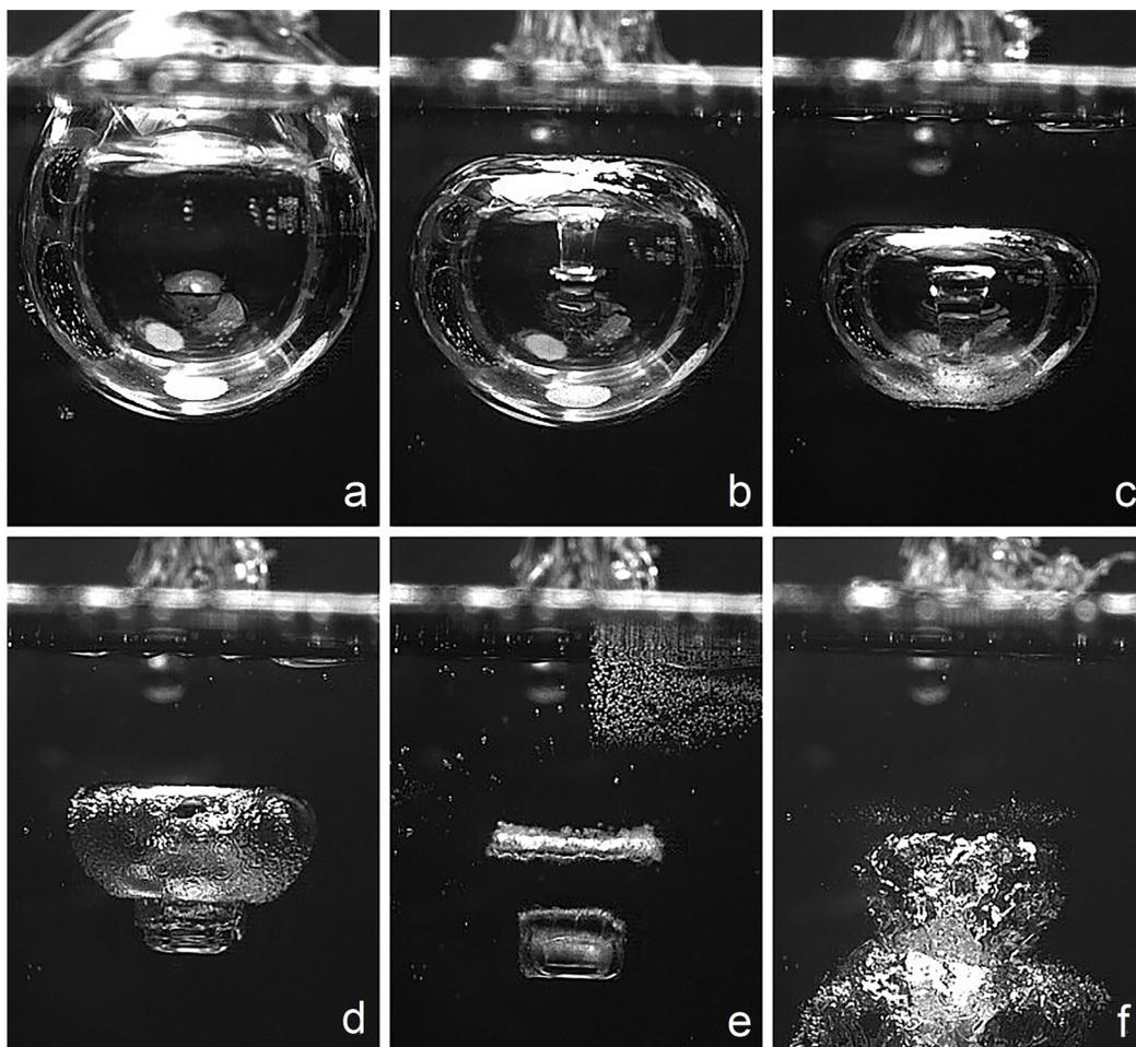
FIG. 1. A centimetric cavitation bubble collapsing in the vicinity of a free surface is pierced by a liquid microjet. The snapshots are shown from instants (a)  $t=0$ , (b)  $t=0.3t_c$ , (c)  $t=0.5t_c$ , (d)  $t=0.7t_c$ , (e)  $t=0.8t_c$ , and (f)  $t=1.3t_c$ , where the Rayleigh collapse time for a spherical bubble ( $t_c=0.915R_{\max}\sqrt{\rho/\Delta p^1}$ ) is used as a reference. Source: APS-DFD (<http://dx.doi.org/10.1103/APS.DFD.2014.GFM.V0084>).
