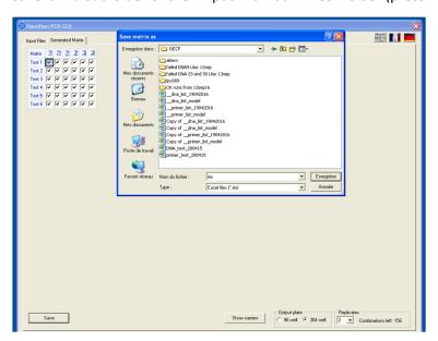
In case you have changed the input files tab after generating a matrix, you may not be able to save. In this happens, close the Hamilton PCR GUI, reopen it and load again the input files.
