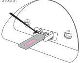
Touch Press to insert new sample; the slide will be automatically pulled into the instrument.
