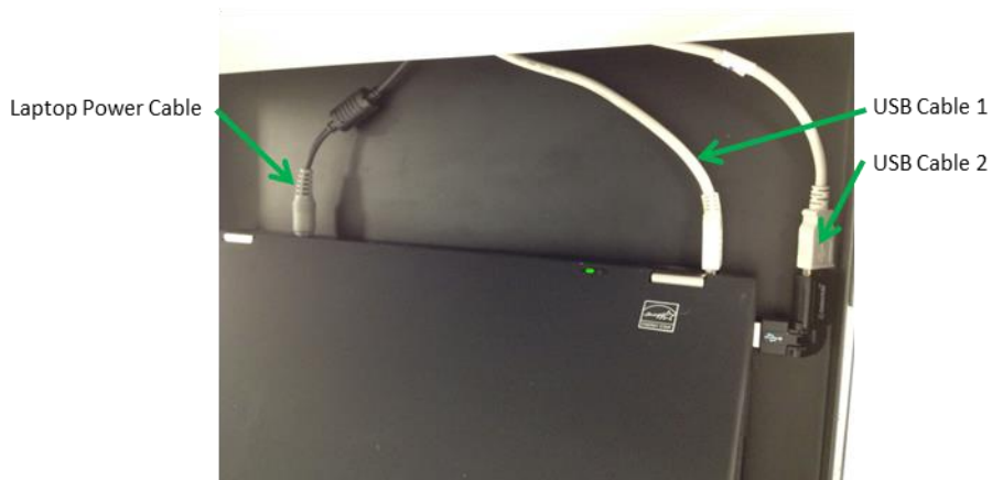
Figure 3-1 – Connections to laptop in rear of laptop drawer. Always keep the power cord plugged in to the laptop. The laptop has two USB cables connected to it. One USB cable is for Ebox communication and the second USB cable is for the serial port hub. The USB port selection for plugging in the USB cables is not critical.
