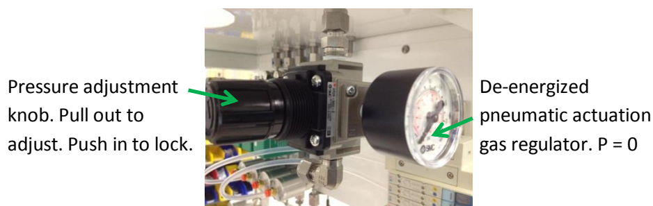
Figure 4-1 – Deenergized pneumatic gas supply
