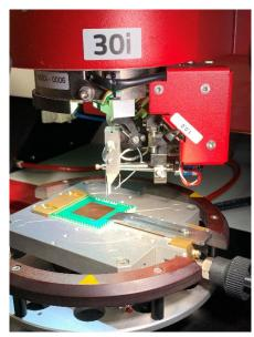
The angle of the bondhead can be modified by changing the "P Position" value with the +/- buttons.
