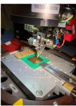
Then, set the current height of the bondhead as the workheight by clicking on the "Apply" button next to the "Workheight 1" and "Workheight 2" fields.
