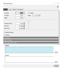
Check the parameters of the bonding for both bonds.
