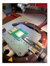
If the sample is small or fragile, there is the possibility to use vacuum instead of the clamp to hold the sample. To do this, switch on the vacuum pump on the left of the tool:
