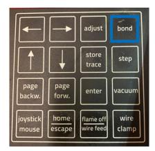
The tool will perform the wire bonding. If successful, wire should be visible at both bond locations.
