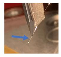
It can also happen that the wire gets out of the tip. This can happen if the parameters of the wire bonding (Bond time, US power, bond force) are too high. In order to place the wire back in the tip, press on the "Feed in position" button on the top bar of the screen
