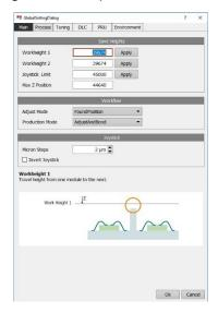
In this step, the workheight of the recipe is set. The workheight is a coordinate along the Z-axis (= height of the bondhead) which should be set few millimetres above the sample. When the tool is initialized, the Z coordinate is set at 0 mm. To set the workheight, the bondhead needs to be lowered until almost reaching the sample.
