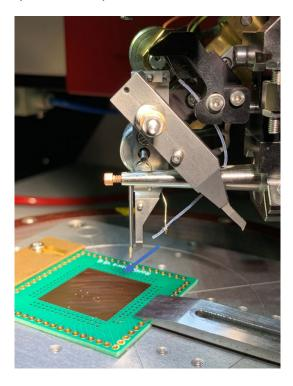
The wire can now be inserted in the tip using a fine tweezer. The wire should be oriented as shown by the blue arrow (45° angle with respect to the tip).
