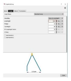
For very short wires, it can be useful to enable the "Use Reverse 1" option to avoid that the first bond detaches while the tip travels towards the second bond.
