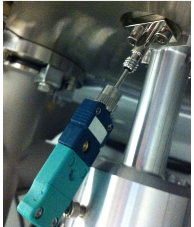
Figure 10 Bottom part of the TC once the connector is moved down of few mm. (NB: the nut must be screwed back in upper position before processing)
