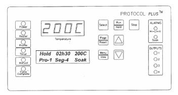
The oven is operated with the PROTOCOL *PLUS* controller.
