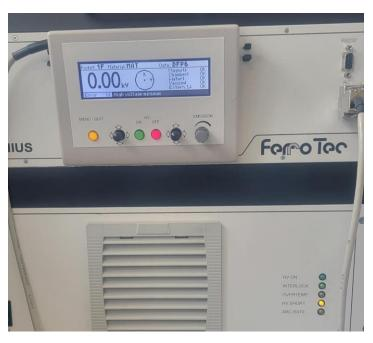
On the remote controller of the e-gun, snap on the front panel of the electrical cabinet, the following alarm is mentioned: *High Voltage Minimum*. The yellow *MENU/QUIT* LED is blinking on the remote controller and HV-Short LED is on the generator.
