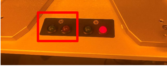
No blinking red LED = cassette missing or wrongly placed
