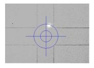
Assuming the equipment was just initialized, the laser spot is located at the (0,0) coordinate of the galvo/piezo stages. Use the joystick to move the sample/wafer so that the laser spot is exactly on top of the (0,0) position of the existing topography.
