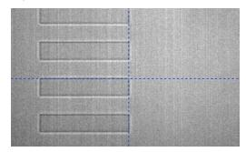
When correctly positioned, click "Get position" to acquire the stage position of the specific marker.
