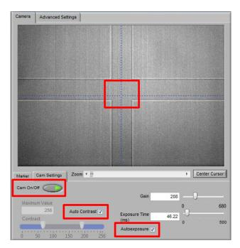
WARNING: Depending on the AxioVision settings, the camera view axes can be inverted in Nanowrite. Make sure to clearly identify your marks!
