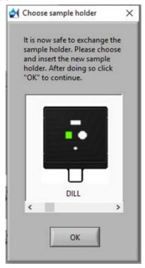
IMPORTANT: Any manipulation on the microscope, i.e. loading/unloading sample holder and mounting/dismounting the objectives, should be done with the "Choose sample holder" window active. Only in this state are the actuators of the piezo-stage deactivated and the stage can move without damage to the equipment! Also, the red LED "BUSY" should be OFF.
