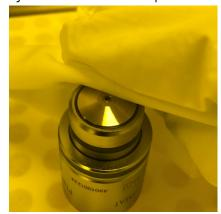
STEP 2: Blow the lens with N2 gun to push the resist/oil from the lens. Wipe around the lens same as described above. Repeat several times.
