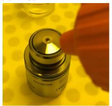
STEP 3: Wrap one tissue around your index, hold the lens firmly and tilt it slightly as shown below.
