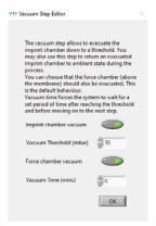
A vacuum step is inserted, when you want to evacuate or ventilate the imprint chamber. All vacuum and overpressures are automatically released at the end of each process run.
