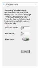
In a hold step, the temperature is kept constant for the set Hold time. The Force Pressure can be set, and you can choose whether the UV source should be on during the hold step.
