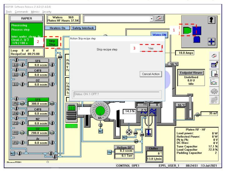
Wait for the **Rapier** module to be **Idle state** after process completion and for the **VCE** to confirm for door opening (1/8 turn counter-clockwise).
