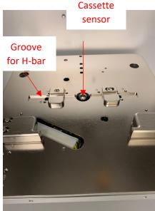
For correct optical detection of the wafer(s), the wafers must be loaded with no flat visible:
