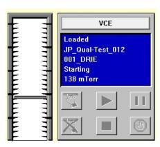
If applicable, pre-cassette, inter-wafer(s) and post-cassette cleaning/conditioning will automatically happen (waferless steps) in the **Rapier** chamber.
