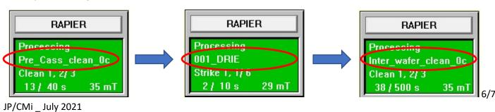
Anytime during process, it is possible to **Skip a Step**: from the main view, **1 Select etch module view**, click the **2 Skip Step** button, and **3 confirm the action**.
