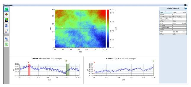
Figure 3.4: Main Display Area for Example PSI Measurement
