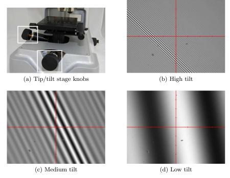
Figure 2.6: Tip/tilt Control & Tilted Fringes
