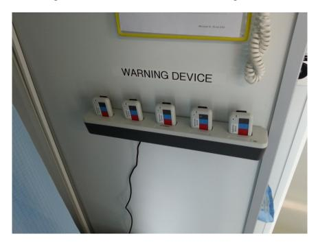
This system is programmed to either detect an action on the red button or to detect a horizontal position.
