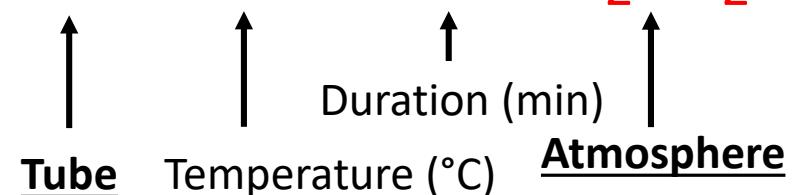
Annealing @ 200 C @ 300 @ 400 during 20min in H<sub>2</sub>/N<sub>2</sub>
