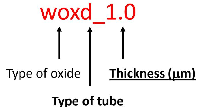
Wet oxide in Wetox tube @ 1050°C during 3 hours
