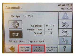
It is recommended to activate the "Vacuum" and check that the wafer chuck vacuum is close to -0.8 Bar.
