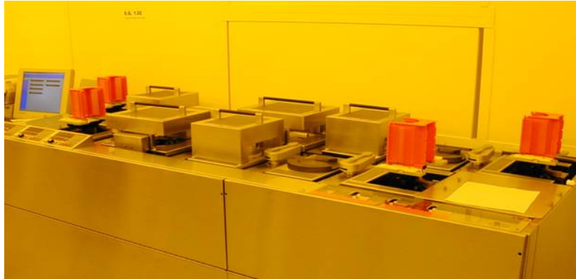
Linear track system for coating (front track) and develop (rear track) of 100mm wafers.
