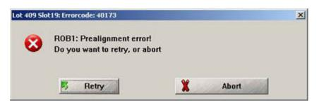
Handling error or restart after "stop". In case a system clean-up is required with the help of the staff (robot mode need to be changed before and after cleaning in supervisor). Pay attention for each step and answer correctly to the questions asked by the system.
