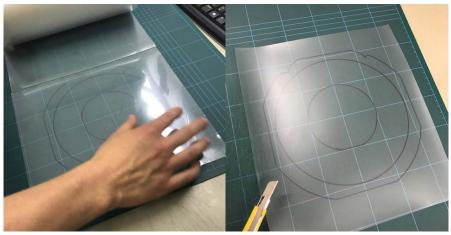
Fetch the roll of UV-tape and cut a piece large enough for the metallic frames. Make sure you place the UV-tape back in its bag as soon as possible and that you properly store it back away from room light !
