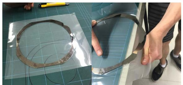
Drop one frame on the UV-tape. While holding the frame flat at the edge of the table, manually stretch (slightly!) the tape from the periphery to have a surface with no wrinkles.
