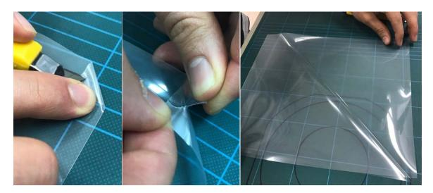
Remove the transparent protective liner. Place the UV-tape with sticky face up !
