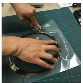
Cut the tape by following the shape of the frame with a cutting blade.
