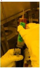
Air is removed from the syringe using the "down arrow" in slow mode and facing the syringe upward. Clean with a paper sheet if any resist spills out.
