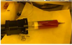
Rotate the syringe ¼ turn to unclamp it from the motor block as shown below.
