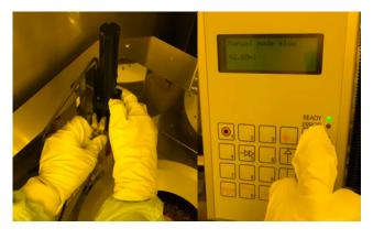
Close the CO2 lateral door and switch back to "Doors Not Accessible" on the UI.
