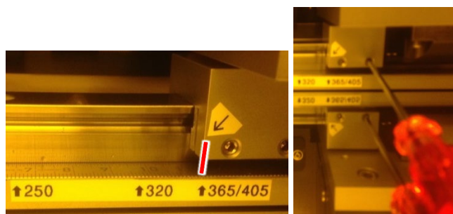
Fig 15: lamp house stopper block locations
