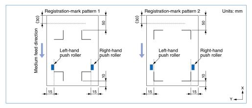
**Note:** The margins in parentheses are the blank margins that must be left between the medium edges and the cutting area in SHEET mode.
