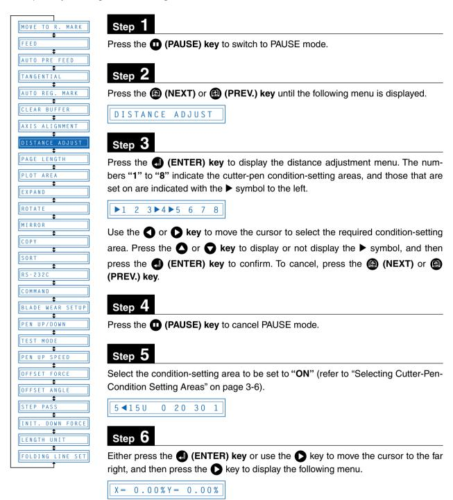
Select "X" or "Y" using the or key. Use the or key to increase or decrease the setting within the range of "-2.00%" to "+2.00%," and then press the (ENTER) key to confirm. If the condition-setting area is set for TANGENTIAL mode, the TANGENTIAL-mode setting will be displayed. Press (ENTER) again. To cancel the selection(s), press the (NEXT) or (PREV.) key.
