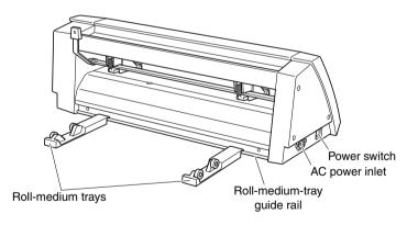
Roll-medium trays : Used to hold a roll medium
