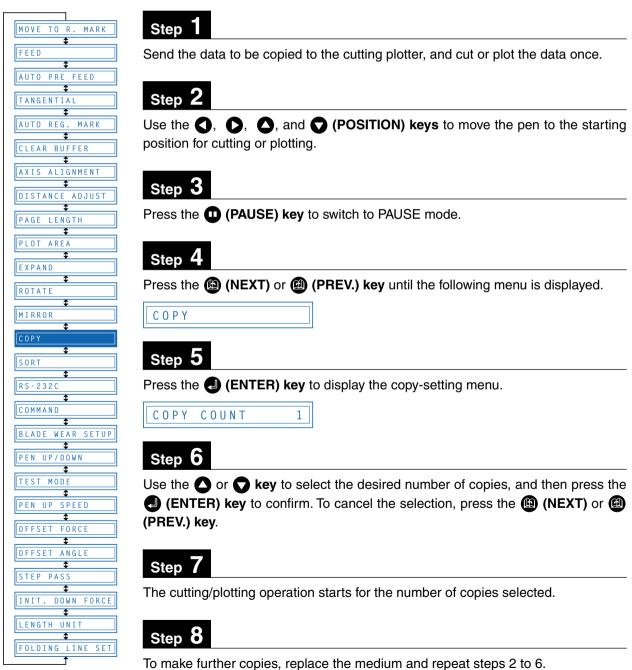
If the data to be copied does not fit within the cutting/plotting area, the following message is displayed in step 5.
