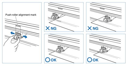
**CAUTION** To move the push rollers, the media set lever must be in the lowered position.
