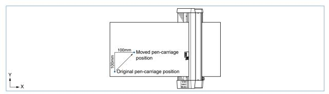
In READY mode, press the **key** while holding down the **(ENTER)** key to move the pen carriage in +100 mm steps along the X- and Y-axes.
