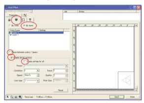
(8) Select the name of the layer where the cutting lines were drawn from the list, and then select "CRP Cut - Vinyl Sticker" from the Preset parameter selections.
