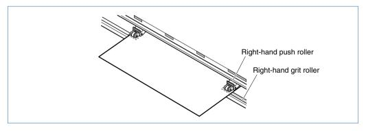
**CAUTION** To move the push rollers, the media set lever must be in the lowered position.
