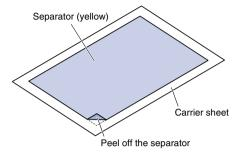
(2) Affix the medium for cutting to the adhesive surface of the carrier sheet, making sure that the edges of the medium are parallel with those of the carrier sheet.
