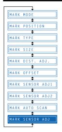
There may be instances when the registration-mark sensor does not function correctly, depending on how it is moved. If this happens, adjusting the sensitivity will enable the sensor to perform detection correctly in most cases.
