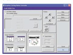
If cutting only will be performed, set the Force, Speed, and other cutting conditions to suit the type of media that you plan to cut (paper or cutting film). Select the media type that you plan to use from the Controller.
