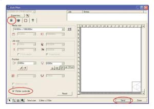
Click the "Send" button to display the "Cutting Plotter Controller".
