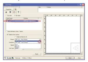
(9) Select the name of the layer where the folding lines were drawn from the list and then select "CRP Fold - Vinyl Sticker" from the Preset parameter selections.
