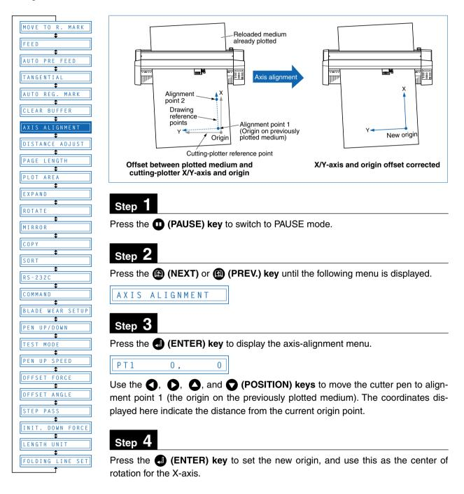
Use the **()**, **()**, and **()** (**POSITION) keys** to move the cutter pen to alignment point 2 (any point on the X-axis for the previously plotted medium). The coordinates displayed here indicate the distance from alignment point 1.
