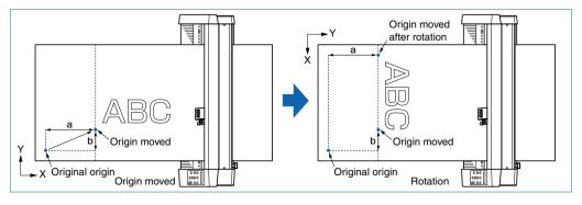
When it is necessary to both move the origin and rotate the coordinate axes, be sure to rotate the coordinate axes first.
