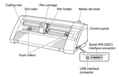
Cutting mat: Cutting or plotting is performed on this mat.Grit roller: Feeds the medium backward or forwardPush rollers: Pushes the medium against the grit rollersPen carriage: Moves the cutter pen to the left and rightPen holder: Holds the cutter pen and moves it up and down
