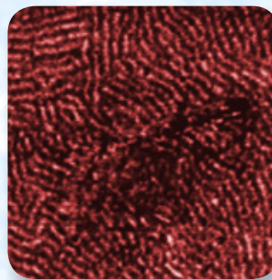
PeakForce TUNA current map reveals current paths in P3HT film. Image size 500 nm. Courtesy of P. Leclere, University of Mons, Belgium.
