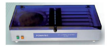
The U-200 from Powatec is a manual UV irradiation system fitted with 31 LED's (310mW @ 365nm). It is used to cure UV-tape to ensure easy and safe removal of thin workpieces.
