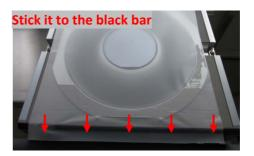
5- Use the manual rolling pad to nicely stick the tape to the wafer + the frame. One single pass is enough. Keep rolling until reaching the roll the tape was initially stuck to.
