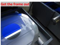
**3-** Stop the machine by pressing on the green button once again. Get the frame out and close the lid. Release the frame first and then get the workpieces. After UV irradiation, the tape is not usable anymore.
