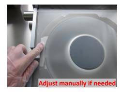
**6-** Lower the cutting system. First, cut the top part of the tape by gently pressing down the blade and going back and forth on the track. Then, cut the whole periphery of the frame using the circular cutting blade.
