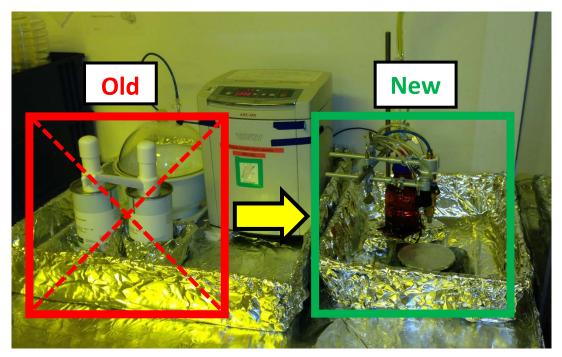
Cans equipped with manual pumps and curing agent bottles will disappear shorty (once empty). Both are replaced by a new system to dispense PDMS & Cross-linker.
