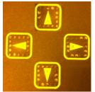
On the MA6 panel: control the fine focus of the left and right objectives with the "TOP SUBSTRATE" knobs.
