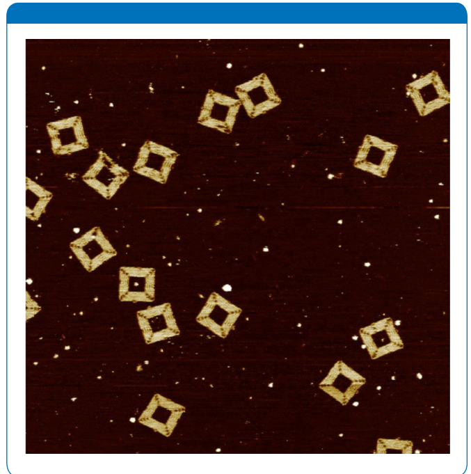
Figure 17. 1µm scan of Origami DNA in buffer solution using ScanAsyst. Single strands of DNA comprising the square structure are clearly discernible.
